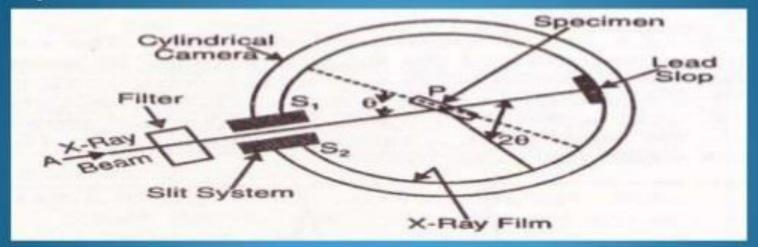
Fine powder is struck on a hair with a gum ,it is suspended vertically in the axis of a cylindrical camera
