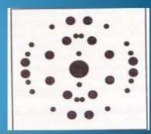
Diffraction pattern of a single crystal of an inorganic sal
